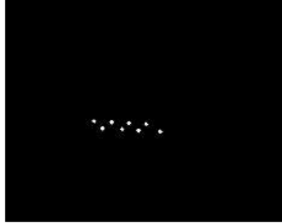
(b) Filtered camera image with programmatically isolated beacon feature points in the image plane.
